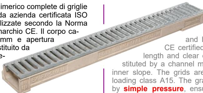
Channels in polymer concrete with grids of galvanized steel produced by certified ISO 9001:2015 company, designed and built according to UNI EN 1433, CE certified. The channel body, 1000mm in length and clear opening **100mm-150mm**, is constituted by a channel made of polymer concrete without inner slope. The grids are made of galvanized steel with loading class A15. The grates are fastened to the channel by **simple pressure**, ensuring the proper stability and silence.
