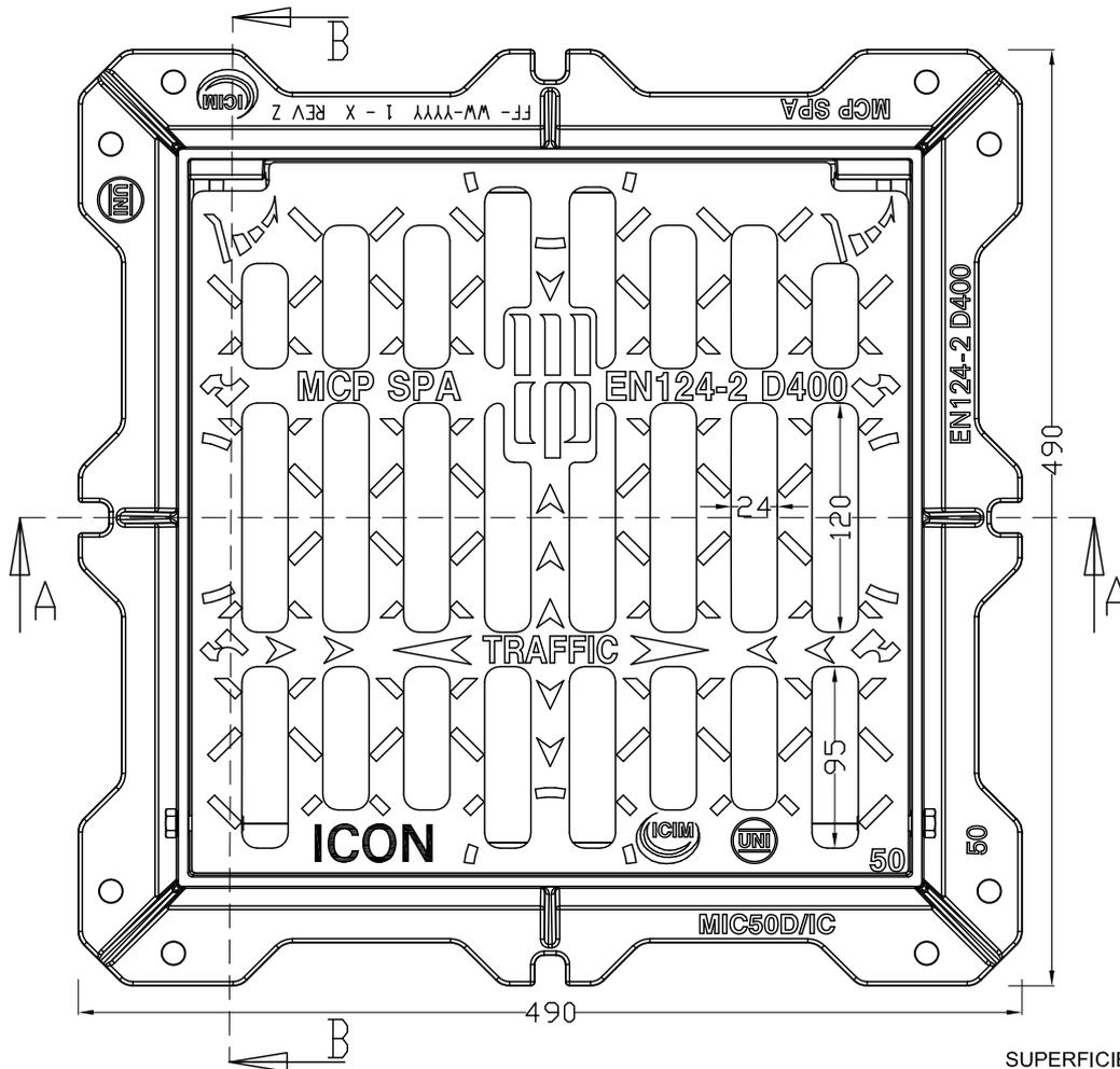
SUPERFICIE DI SCARICO = 5.07dm<sup>2</sup>
